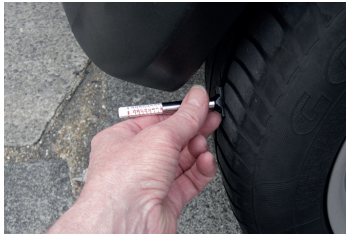
The minimum legal tread depth for a car tyre is 1.6mm.
